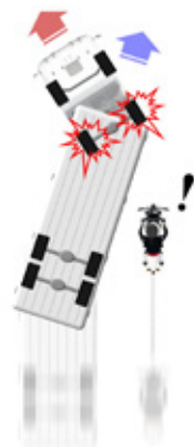
拖車頭後輪鎖死 (拖車頭車尾偏擺)
